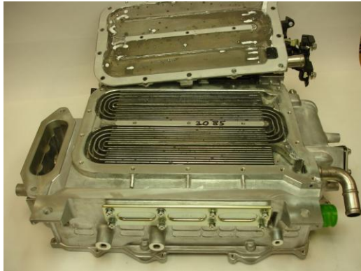
Heat sink used in Nissan Leaf (source : ORNL report)
