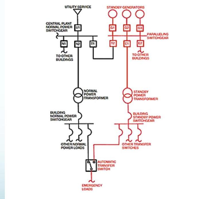
The concept connects the *utility* and the *emergency* sources for paralleling, and, it can maintain voltage on the *emergency* distribution system when the generator source is not on line.
