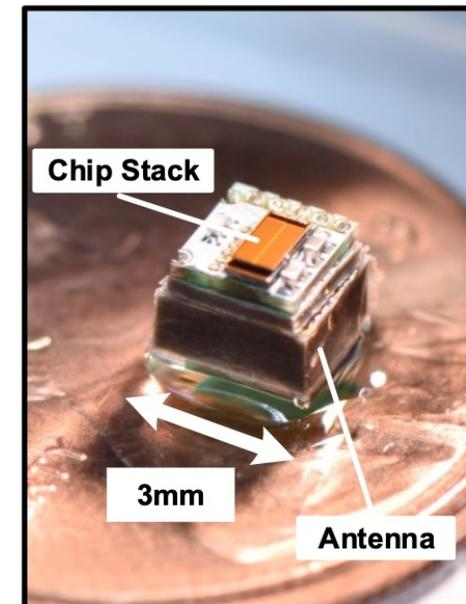
[1] A Fully Integrated 0.2V 802.11ba Wake-Up Receiver with -91.5dBm
