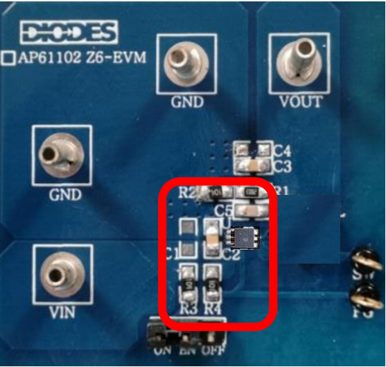
Existing 1A DC/DC AP61102 w/ integrated inductor in 1.8x1.8 mm package
