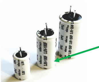
Lithium supercapacitors [Source: Vinatech]
