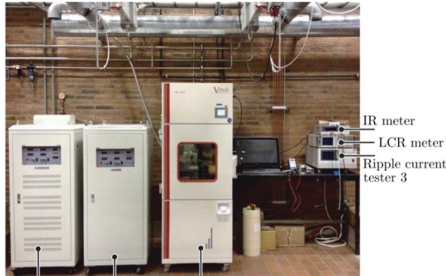
Ripple current tester 1 Ripple current tester 2 Climatic chamber Capacitor degradation testing setup
