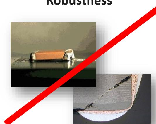
Polymer can sustain mechanical stress where MLCC fails
