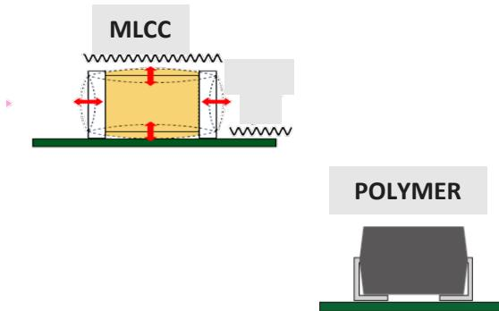
Polymer will not suffer from piezo effect when a rectangular shaped signal is applied
